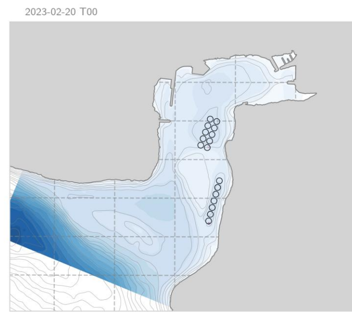
LADiM model setup: Forcing: farcoast26m_bjsj_run5_version3_his_0001.nc IBM module: ladim_plugins.sedimentation, particle lifespan: 14.0 days, Taucrit: 0.018 Model timestep: 60 s, output: 24 h
